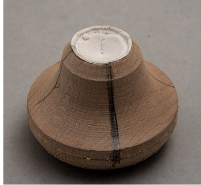
Figure # 14: The completed Cup Aux Chuck.
