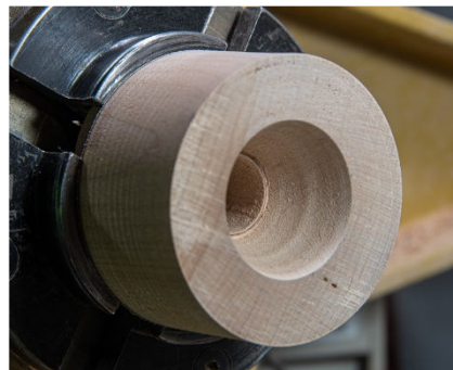
Figure #10: Turn the sloped inside wall of the chuck.
