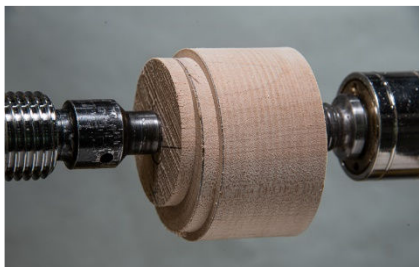
Figure #5: Mount the blank by the offset dimples.
