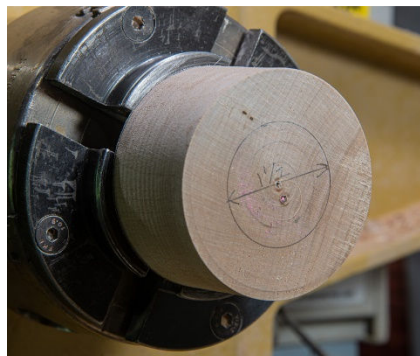
Figure #7: Draw a 1-1/2" circle on the face of the blank.
