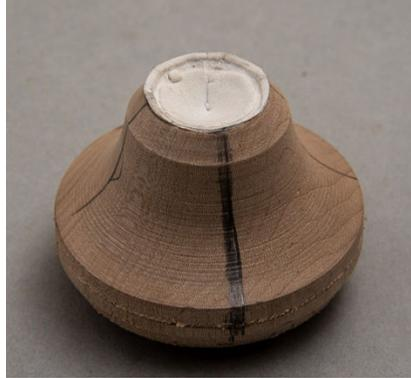
Figure # 14: The completed Cup Aux Chuck.
