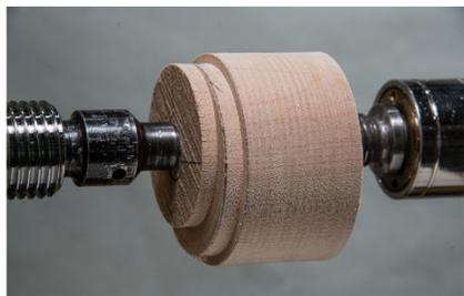
Figure #6: Turn a 2" tenon just less than 1/4" deep.
