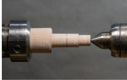
Figure #5: Turn the last 1/2" of the mandrel to 1/2" diameter.
