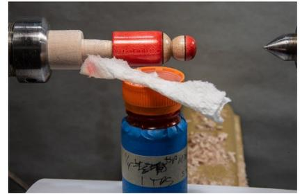
Figure #33: Apply friction polish.
