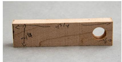
Figure #9: Drill a 5/8" hole near one end.
