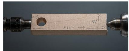
Figure #10: Mount the Removal Tool blank between centers.
