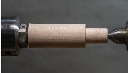
Figure #3: Mount the Mandrel blank between centers and turn a 3/4" diameter mounting tenon.
