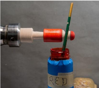
Figure #29: Apply the dye.
