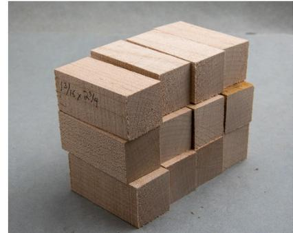
Figure #1: 12 blanks cut to 1-3/16" x 1-3/16" x 2-3/4"
