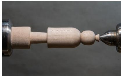
Figure #24: Shape the shoulders and head.
