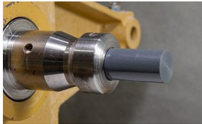
Figure #8: Turn the face of the body flat and chamfer the rim.
