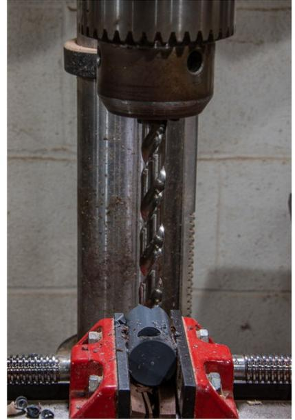
Figure #10: Drill through the body with a 1/2" drill bit.
