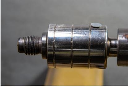
Figure #12: Insert a roofing nail to lock the tailstock center rotation.
