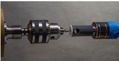
Figure #14: Drill an axial hole through the foam and body face.
