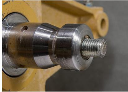
Figure #7: Mount 3/4x10 threaded rod in a chuck.
