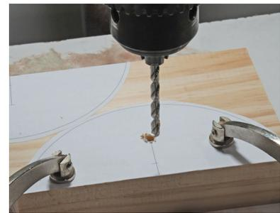
Fig02: Drilling holes for the mounting screws in the wooden jaws.
