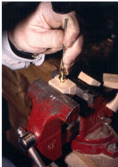
To drill the hole to insert the wire I transfer the detachable mechanism and the wood blocks to my cross-vise and insert a micro-drilling fixture into the chuck of the drill press. That's not to say you need to have these tools, it only means that my tool fetish got the better of me. You could probably get good results with a drill press and any means to hold the mechanism, or even a hand drill. These fancy tools just make it
