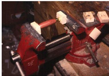
Unscrew the magnifying glass bezel from the mount and press the mount into the tube. Be sure to mount it in the smaller diameter end. Then take the detachable mechanism apart and mount the female half in the other end of the tube. At this point you can re-attach the magnifier bezel to the mount.
