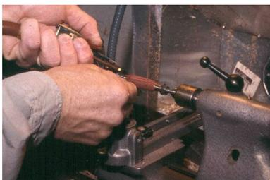
In Figure 6 I'm applying a friction polish:
