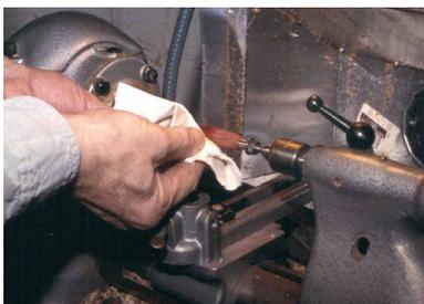
Once you're done turning the blank, remove it from the lathe.
