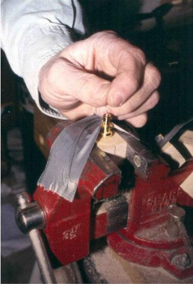
It didn't feel real tight, so I added a little extra glue by dipping a small wood scrap into the glue to controllably transfer some more glue around the wire. Then I sprayed a little accelerator onto the glue to finish the job. If you can only find a #60 drill you may have better luck if you use polyurethane glue, which fills gaps better.
