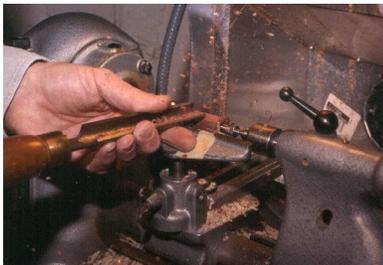
Figure 5 shows sanding the blank smooth:
