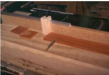
This time I cut the board into squares, then drilled the hole for mounting the shaft on my drill press (a drill press is more or less a hand drill on steroids). By cutting the blank square first, I could use a jig to accurately and quickly locate the hole for drilling
