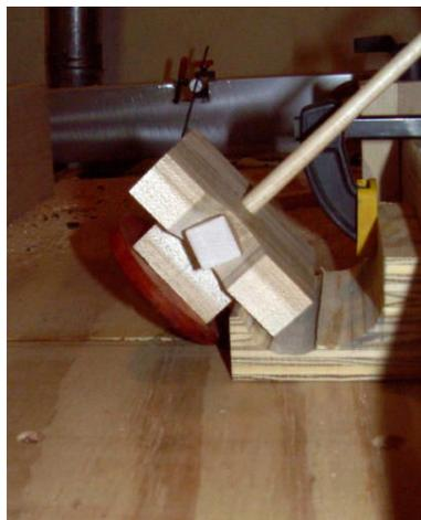
This is an even newer notch jig. This one locks on the shaft with a wooden screw, and the notch depth doesn't vary with minor changes in whorl size, which was a problem with the last jig. Using a different saw blade flattened out the bottom of the notch too.
