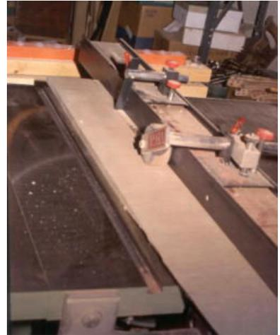
The last step is to cross cut the strips into shaft blanks 10 1/2 inches (27cm) long.
