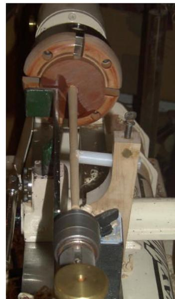
[This picture shows a handy idea I've come up with since the article was written. It's a quick mount center steady that makes it easier to turn the long thin shaft without burning my fingers.](#)
