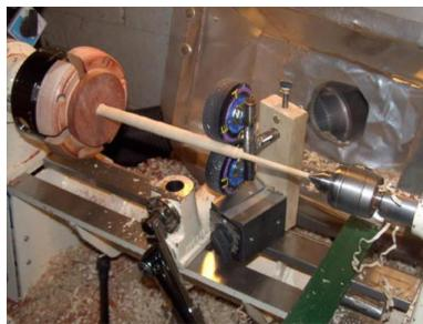
Steadying a drop spindle shaft.
