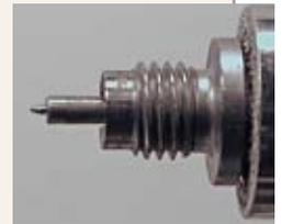
After filing a tapered dowel pin into a limited penetration center.
