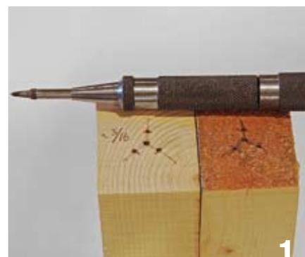
1 With a centerpunch, mark offset centers on the headstock end of the turning square.
