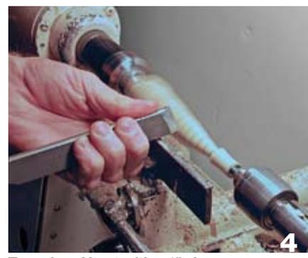
4 To make a V-cut with a 1" skew, use an underhand grip with your index finger hooked under the tool rest to anchor your hand.
