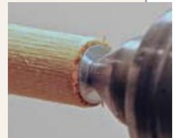
Use a small washer to prevent the tailstock from penetrating too far and splitting the soft pine.
