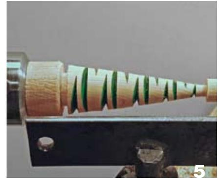
Skim the surface of the tree to remove excess paint and pencil lines.
