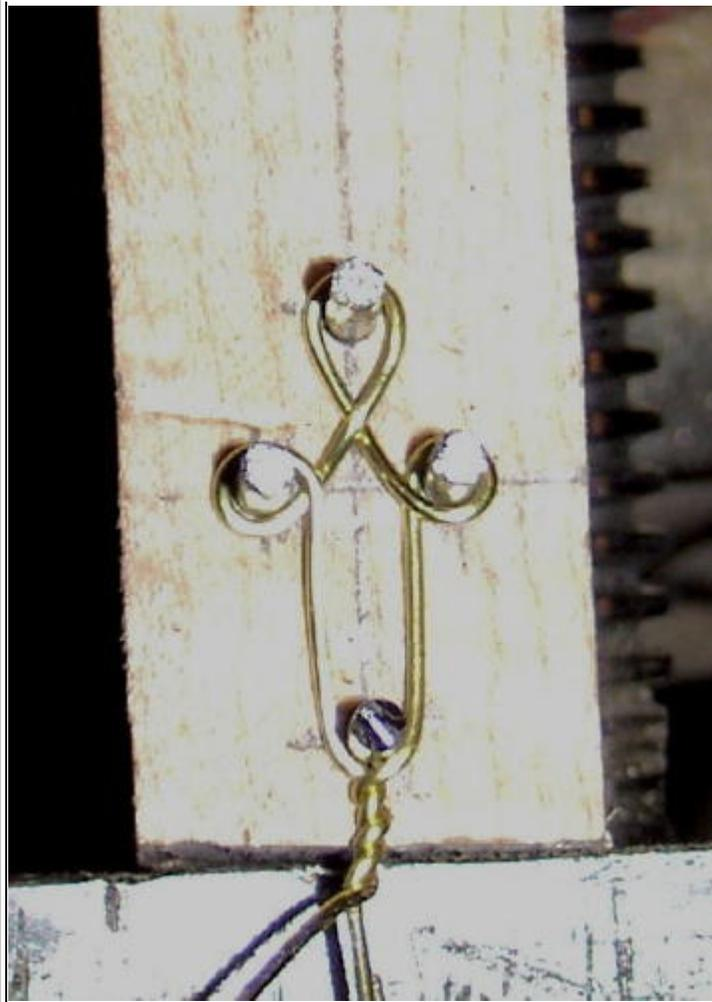
The wire bending form. I start at the bottom, going around each nail in counter-clockwise order, then twisting to tighten up.
